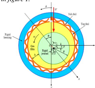
Fig. 1 First generation gas foil bearing cross-section schematic, and gas-film and bump foil structure models.
