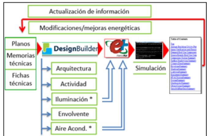
Fig. 3. Flow diagram for energy modeling.
