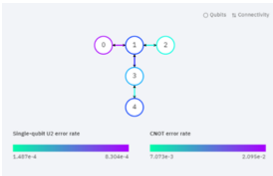
Figura 8. Calibration scheme for IBM Yorktown quantum processor
